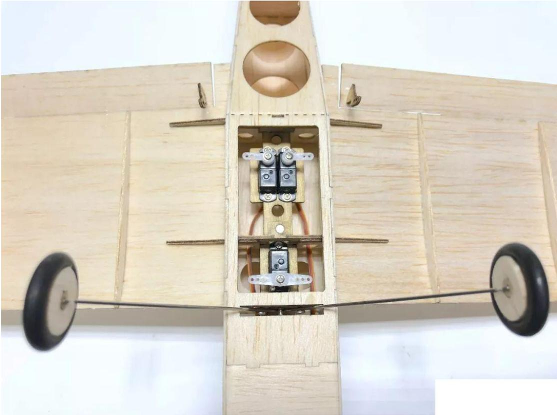
52. Connect the pushrod clips & pushrods with heat shrinkable tube and fix them with glue.
