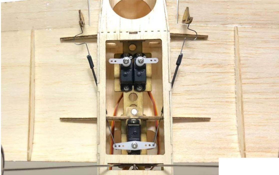
54. Connect the pushrod clips & pushrods with heat shrinkable tube and fix them with glue.
