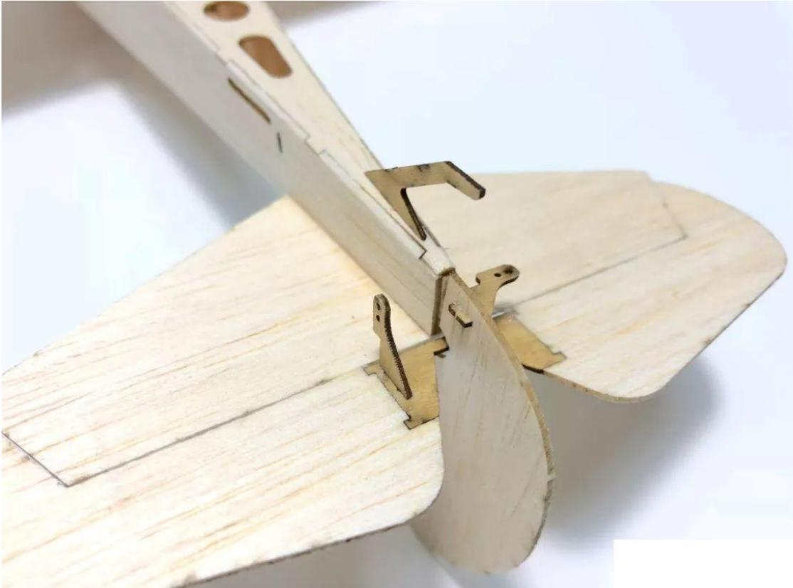
45. Installation of the control horns.
