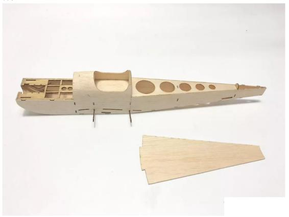
18. When the balsa is too difficult to bend, wipe the outer surface with a wet cloth.
