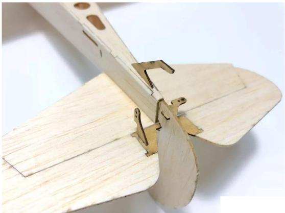
45. Installation of the control horns.
