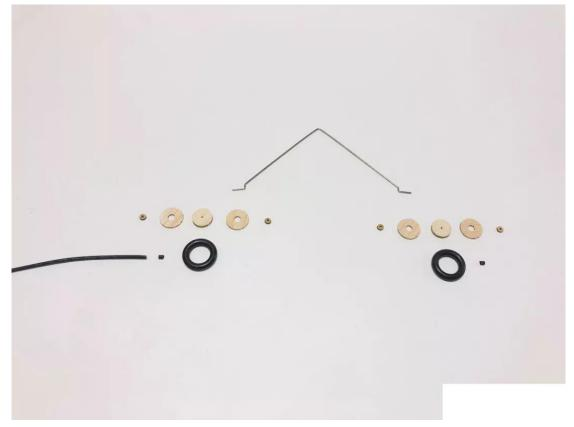
43. Use heat shrinkable tube to hold the wheels.
