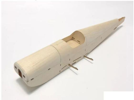
29. Insert the windshield fixing bar into the fixing hole of the fuselage and glue it from inside.
