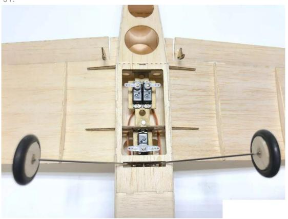
52. Connect the pushrod clips & pushrods with heat shrinkable tube and fix them with glue.
