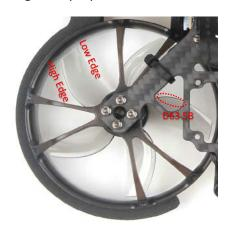
If you look at a prop blade, you will see that there is a *high* edge and a *low* edge. The blade is designed to spin in the direction that the *high* edge is facing.
