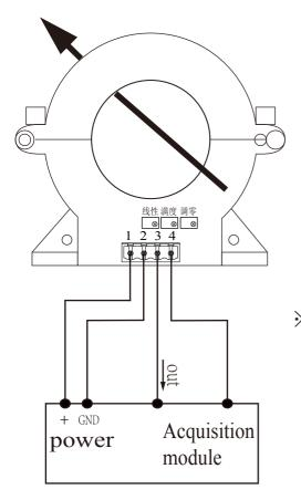
Crimping terminal fast plug2EDG-5.08-4p spacing 5.08mm
