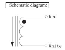
Specifications of lead wire:  $0.3 \text{ mm}^2$ red and white soft line The length of lead wire:  $40 \text{ cm} \sim 45 \text{ cm}$ Color of lead wire: Red, White
