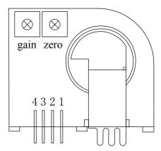
String the sensor bus into the circuit under test
