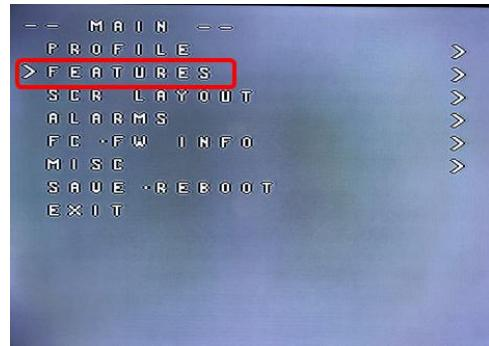
If you are using a video transmitter that supports remote configuration, enter the “Features” menu to configure the vTX. From there, enter either “VTX SA” if you are using SmartAudio (TBS Unify) or “VTX TR” if you are using IRC Tramp Telemetry.
