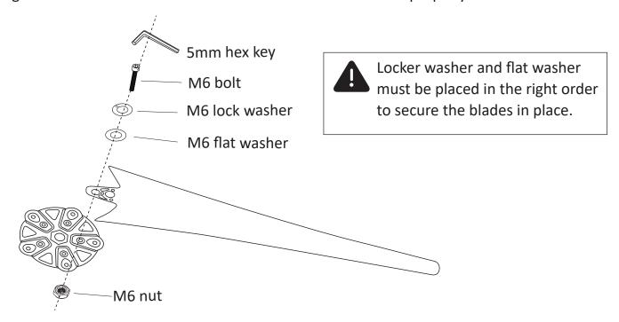
Step 6: Slide the blade assembly onto the rotor shaft and place the lock washer and lock nut on the shaft. Make sure the lock washer is right next to the lock nut.
