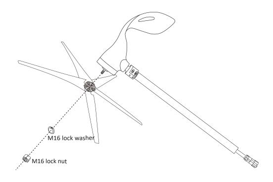
Step 7: Insert the 8mm hex key into the rotor shaft. Hold the blade assembly and tighten the M16 nut by turning the 8mm hex key counter clockwise. If needed, please use the extender (not included) to extend 8mm hex key to tighten the lock nut. Finally, spin the blades slowly to be sure they turn freely and the hub does move in along the rotor shaft.
