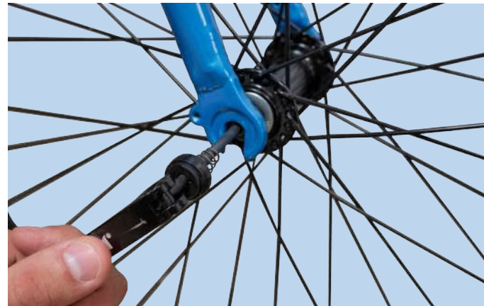
Figure 10. Inserting the Quick Release Skewer
