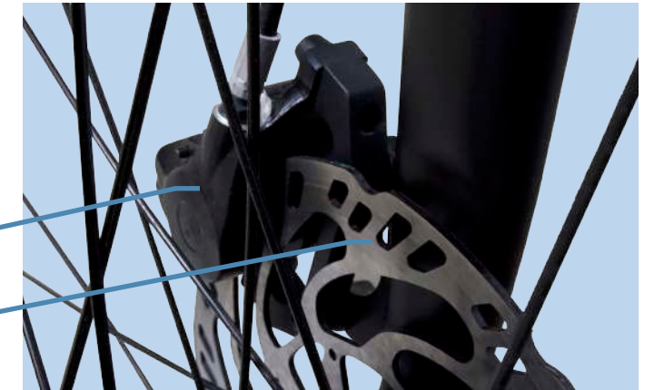
Figure 7. Sliding the Caliper onto the Rotor
