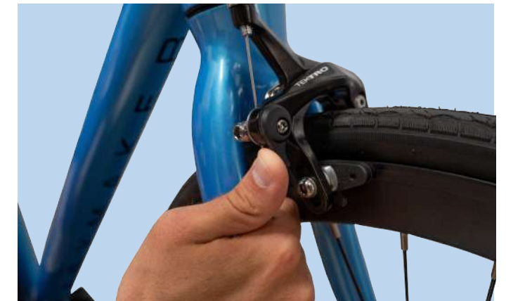
Figure 9. Locking the C-Brakes on Standard Model
