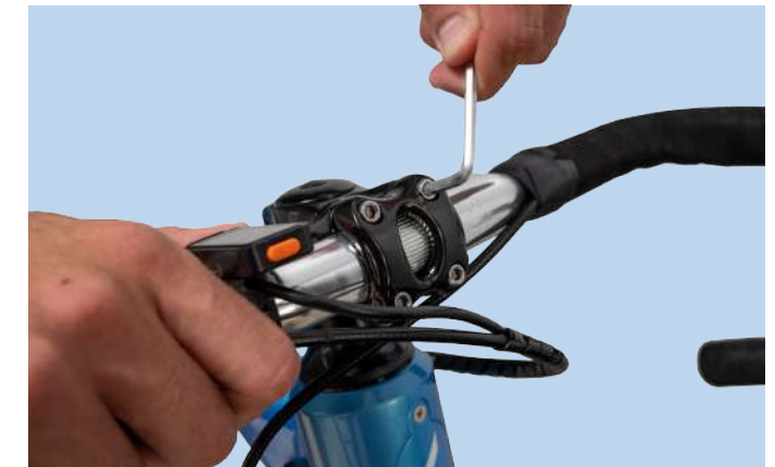
Figure 2. Tightening Stem Plate Bolts
