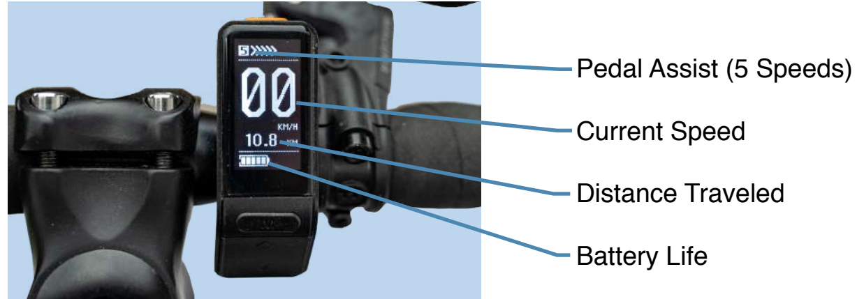
Figure 22. Checking the LCD Display
