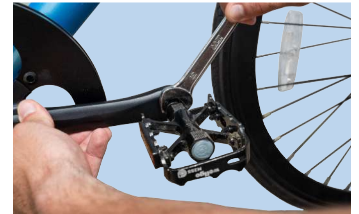
Figure 14. Attaching Pedal to Crank
