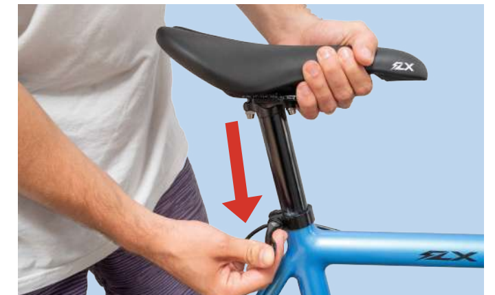
Figure 15. Dropping Seat into Bike
