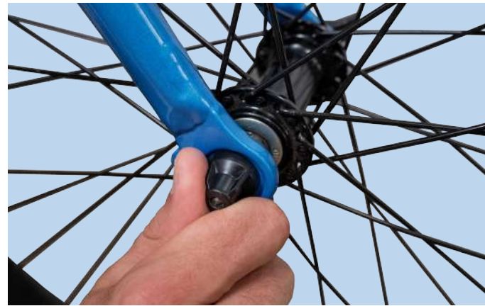
Figure 11. Tightening Quick Release Skewer
