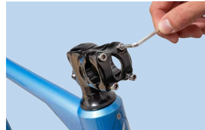
Figure 1. Stem Plate Bolt Removal
