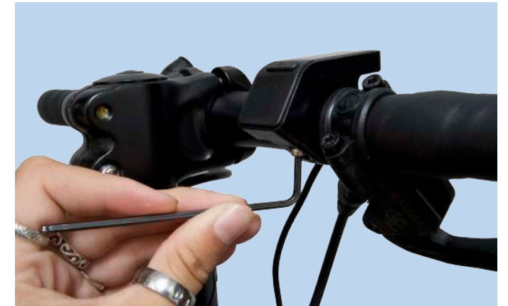
Figure 19. Tightening the LDC Display
