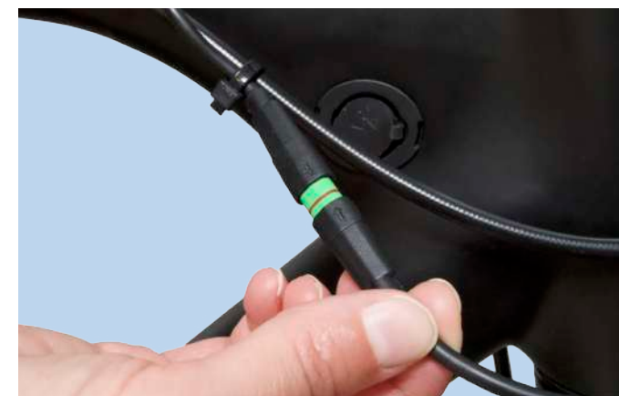
Figure 3. Connecting the LCD cables
