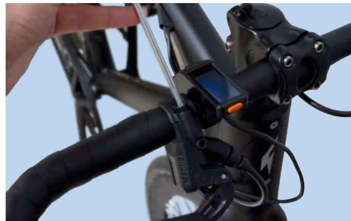
Figure 17. Attaching the Brake Levers
