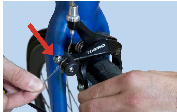
Figure 6. Re-Tightening the Brakes
