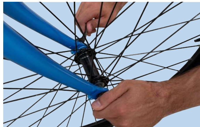
Figure 12. Testing Wheel Tension
