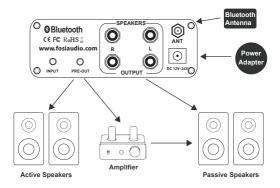
Note: You don't need to connect all the outputs. You can connect 2 passive speakers only. Or you can connect it to the pre-out as a preamplifier. And you can connect all the outputs simultaneously.
