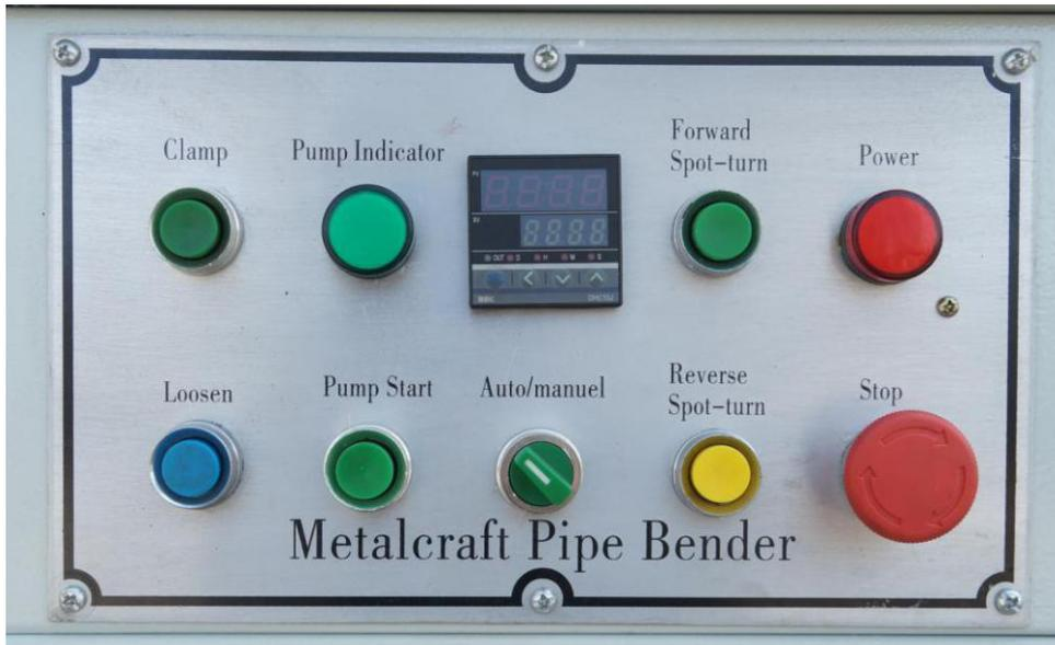
(1) Clamp: Work at Manual mode, press on this button to clamp the workpiece.
