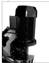
The gear box requires periodic changing of oil. The oil must be changed by the first 6 months of a new machine and every year there after.
