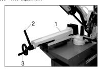
Clamping the Work Piece
