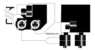
In case the blade needs to be replaced ,make sure to always install 0.9mm thick blades for which the blade guide bearing have been adjusted, in the case of toothed
