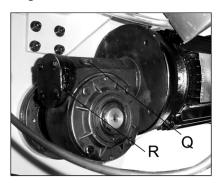
The gear box requires periodic changing of oil. The oil must be changed by the first 6 months of a new machine and every year thereafter.
