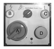
A:Main connect switch B:Power ON indicator light
