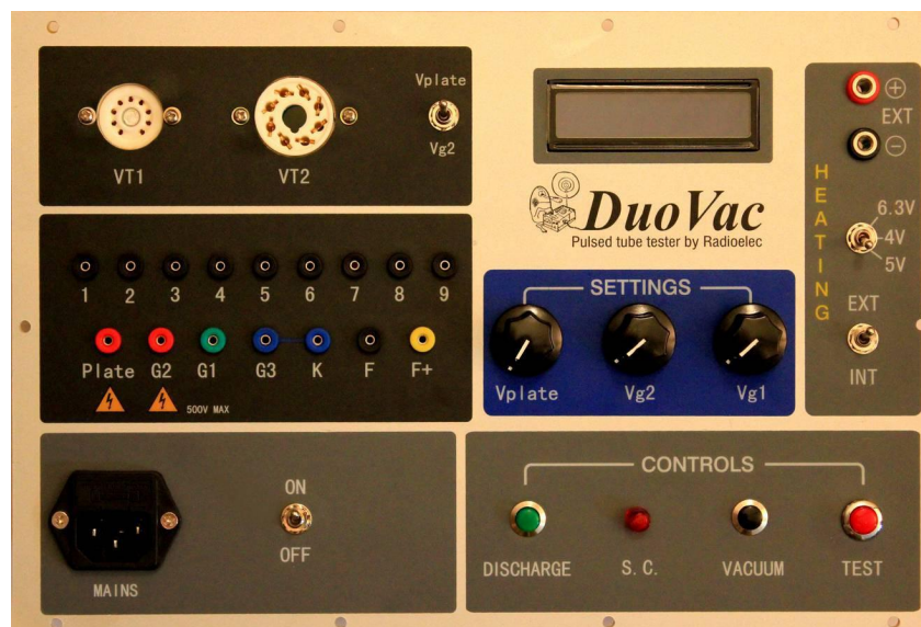
Example of a ready to use tube tester made with the DuoKit module.
