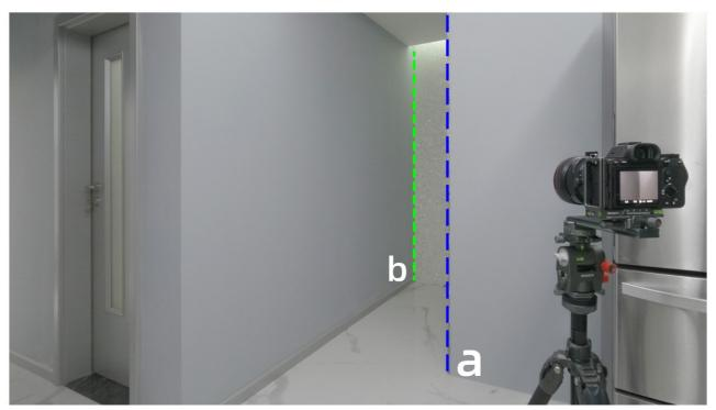
3.3 Loosen the pan lock on the CAP-360 and pan the camera to see if the vertical lines become separated and move relative to each other. Panning to the opposite direction will reverse the apparent shift of vertical lines.
