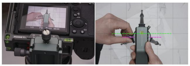
P.S. If you have a **TSE FRAME** and want to shoot panorama with your tilt-shift lens, the step 1/2/3 and 7/8 are not needed. Simply fixing the **TSE FRAME** nodal plate directly on the the upper rotator (CAP-360) and align the marker to the centre of the clamp. Then, align the centre mark of the main bracket to the centre mark on the lower CAP-360, the node aligning is all set.
