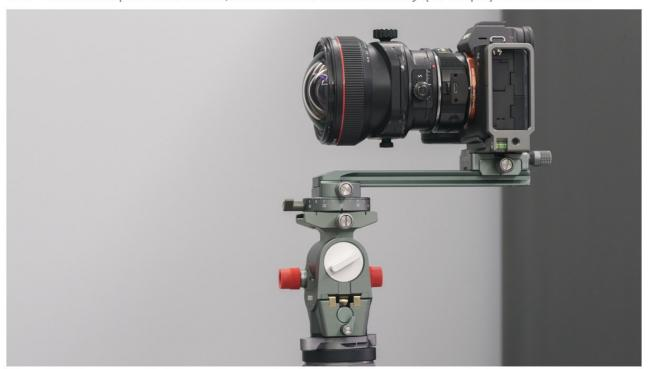
3.2 Look for a vertical line (a door frame or the edge of a cupboard) some 1.5m from the lens that can be lined up with another vertical line some distance further away. A door/window frame can be useful in this respect. Point the camera directly at the near vertical line and note the alignment with the distant feature.
