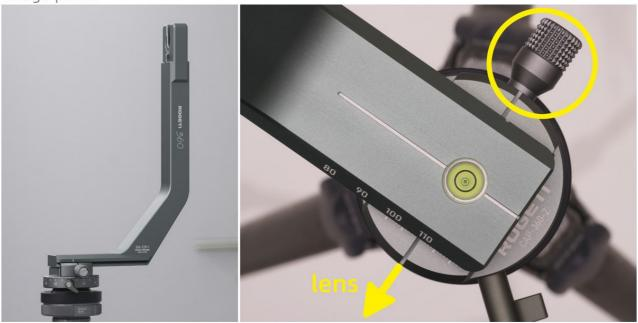
6. Place the upper assembly on the main bracket (360-220) with the pan-lock knob of the upper rotator (CAP-360) facing upward, secure with the large mounting knob when the rotator (CAP-360) is fully slid into place at the top of the main bracket.
