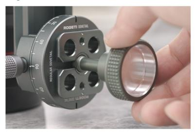
5. Mount another rotator (CAP-360) onto the tripod. Install the main bracket (360-220) onto the rotator. Level the tripod according to the bubble level. Note: When installing the main bracket, having the device-lock knob of the CAP-360 on the opposite side of the lens will avoid the knob appearing in the panoramic
