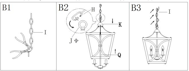
Step B1: By measuring, determine the correct number of links needed for proper hanging height. Using the chain pliers, disconnect and discard the unwanted part.
