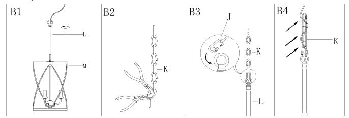
Step B1: Thread the tube (L)onto the fixture body (M) till tight .
