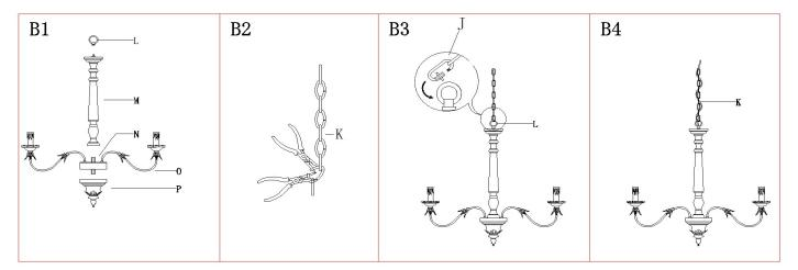
Step B1: Thread the post (M)onto the fixture body (N) till snug; thread the loop (L)onto the post (M) till snug; thread the bottom trim (P)onto the bottom of fixture body (N) till snug.
