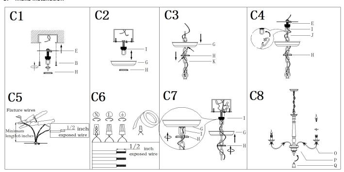
Step C1: .Attach the single bar (E) to outlet box with mounting screws (B). The side of single bar marked "GND" must face out Unscrew the collar ring (H) from the collar loop
