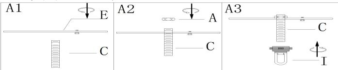
Step A1: Thread the single bar(E) onto nipple (C), At this point need note that: the side of single bar(E) marked "GND" must face to the down.
