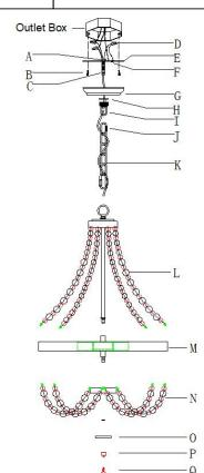
Step A2:Thread the hex nut (A)onto the nipple (C) till snug.
