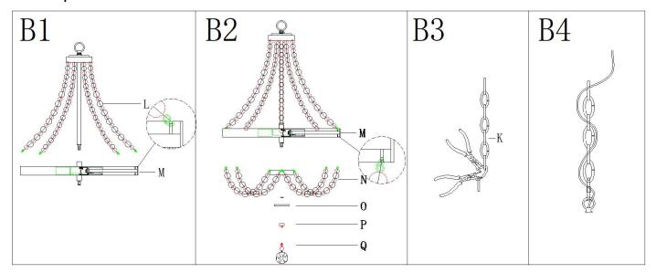
Step B1: Thread the fixture (M)onto the threaded nipple on the fixture body (M)
