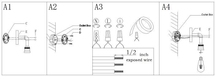
Step A1: Unscrew the knob nuts(F) from back plate(E) then gently remove mounting plate (B)
