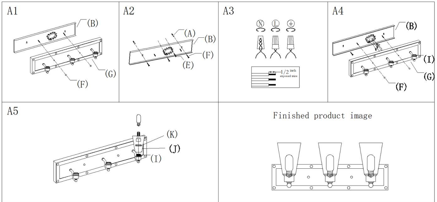
Step A1: Unscrew the knob nut(F) from back plate(G) then gently remove mounting plate (B)
