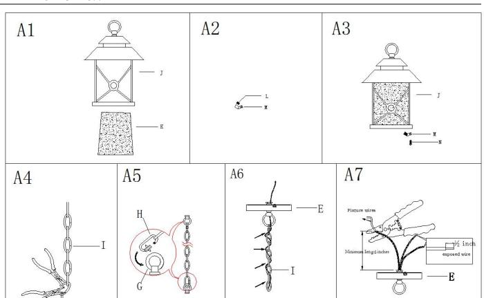
Step A1: Carefully place glass (K) into the fixture frame (J). At this point, the glass has two different sizes, the bigger end of glass must be faced down.
