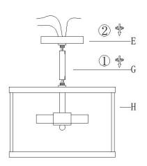
6. Install bulb (Not included. Please do not exceed the maximum capacity recommended on the socket.)
