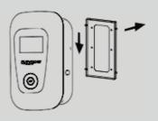
4. Open the rear cover panel and connect according to the markings.
