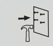
2. Hammer the M8\*80 expansion screw tube into the wall hole.
