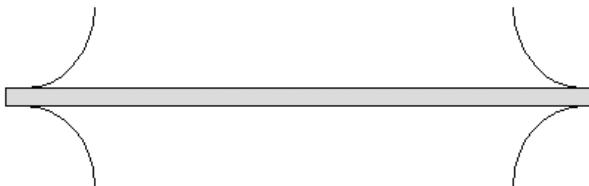
Bad positioning, flap seals closed at end of gel, current cannot get to gel.
