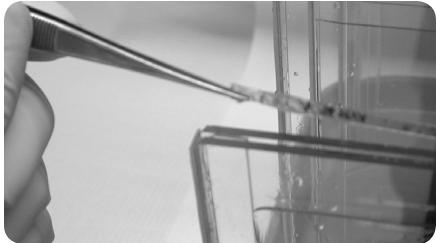
**Fig 17.** Applying IPG strip to second dimension gel.
