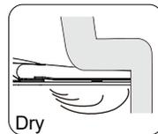
② In the process of drying, press the "🌸" button to adjust the air temperature, and the indicator light will light up to display the wind temperature range. When the indicator light is not on, it is 0 grade (normal temperature range), and the range adjustment mode is 0-5 grade in turn.
