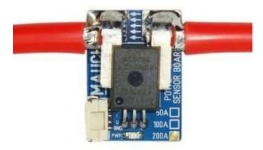
The PL-xxx boards are based on the famous Allegro ACS758 (or 770) hall current sensors, ACS758-050U for the 50A version, ACS758-100U for the 100A version and ACS770-250U for the 200A version. The electronic on the board is powered by an PL - Series or PC - Series BEC and the offset shifting is realized by an OP from Microchip specially designed for microprocessors analog inputs.
