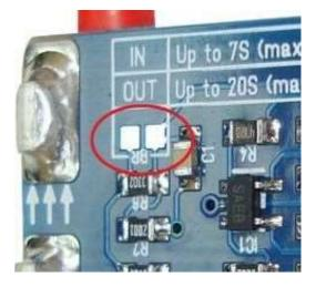
First select the correct voltage measurement range according to your used main battery.
