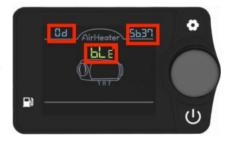
② Connect to the mobile phone via Bluetooth: Click on the Bluetooth symbol "≯" in the upper right corner, find the corresponding local Bluetooth number: BYD + MAC address of the Bluetooth device + 4 digits (4 digits is shown in the upper right corner of the LCD switch controller screen, refer to the picture above), then click on the Bluetooth number to connect, press "adjusting knob" exit this interface.
