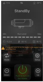
④ Click "Mode" button to switch the level mode or smart mode (temperature control mode), then Click "⊕"/⊙" button to increase or decrease the level value( level 1-10) / temperature value(8°°C ~ 36°°C).
