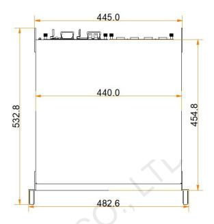
Tolerance: ±0.5 Unit: mm
