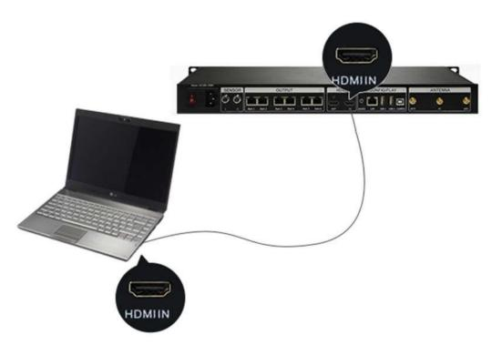
**Note:** C7 will automatically switch to play sync signal program when an external HDMI signal input is detected. You can press **[ Input Switch ]** button to return async signal program playing.
