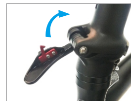
3. Flip the riser over and lock the safety folding buckle
