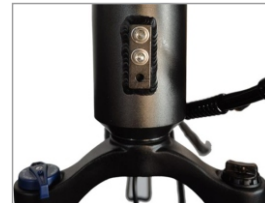
6. There are 3 holes in total, please select the top 2 holes for installation, as shown in the figure
