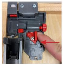
3 Squeeze release tabs and remove drawer box from runners.
