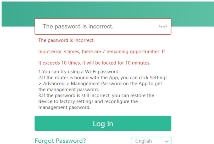
If you forget the IP address or password, hold down the **Reset** button for more than 10 seconds to restore factory settings. After restoration, you can use the default IP address and password to log in.
