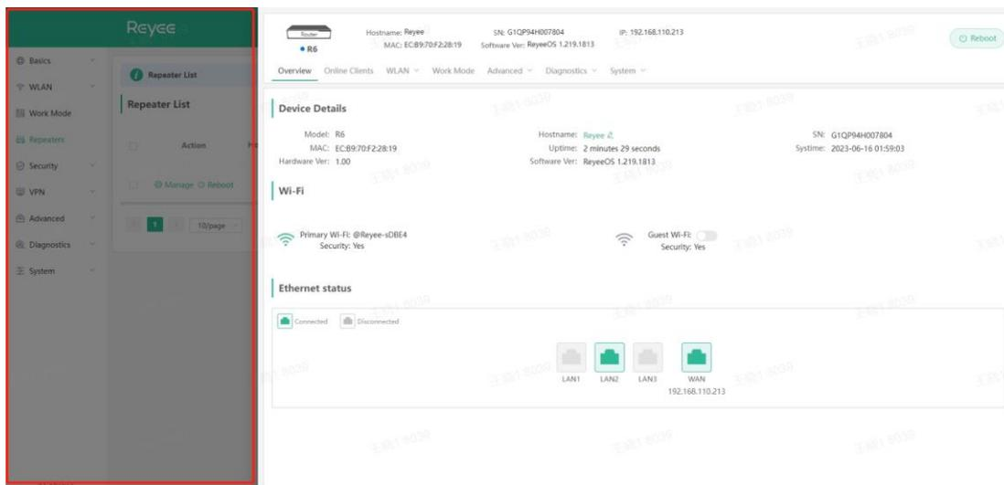
To log in to the web management system of the secondary router directly, you need to know its IP address. Connect your mobile phone or computer to the Wi-Fi network broadcast by the router. Enter the IP address of the secondary router in the address bar of the browser to access the web management system.
