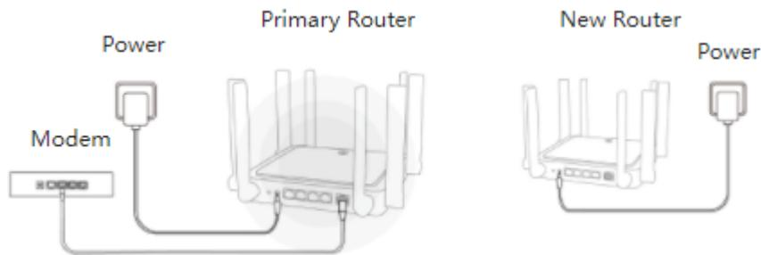
(3) Press the Reyee Mesh button on the primary router.
