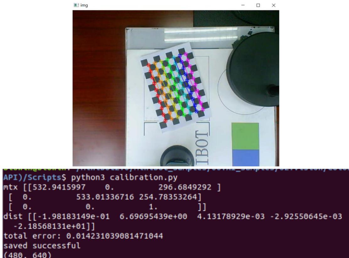
7. Run 4.FigureOutMapParam.py on the terminal to make the entire checkerboard appear in the image display window. Click the image display window, press "Space" to calculate the length of the checkerboard, if "saved successful" appears, the calculation is successful, and press "Esc" to end;
