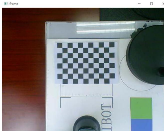
4. Click on the image display window and press the "S" key to save the image. Enter the number "1" on the output terminal, name the photo just taken, and press the "Enter" key to end the saving of the first photo;
