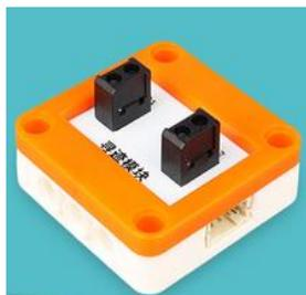
**Line patrol sensor:** It is used to detect black and white lines.
