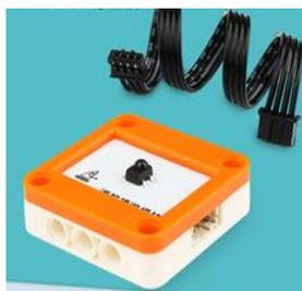
**Infrared remote receiving sensor:** It is used to receive button information of the infrared remote control.
