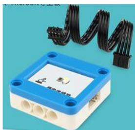
**Color sensor:** It is used to detect different colors and feedback results.
