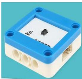
**Gesture sensor:** It is used to recognize gesture movements such as up, down, left, right, front and back.
