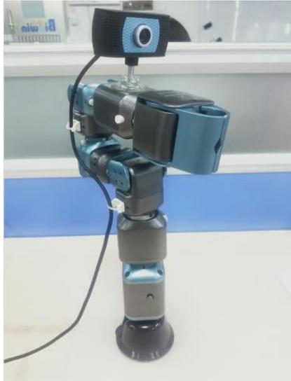
The camera is fixed at the end of the T module. First, the camera and the camera fasteners of T module need to be fastened with M6 bolts, and then the camera is fixed at the end of the T module through the unified two-leaf quick interface, as shown in the figure:
