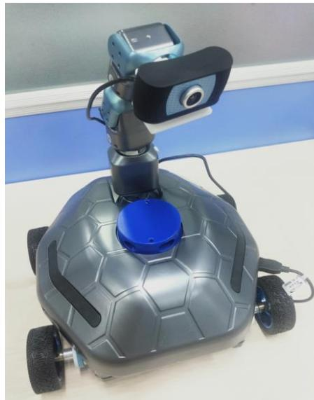
If the sensor needs to be installed on the P module, the sensor fixing plate of the P module needs to be fixed to the top interface of the P module through the unified two-leaf quick interface, and then the sensor is fixed to the sensor fixing piece of the P module through Lego accessories, as shown in the figure:
