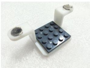
**The sensor fixing plate of the M module:** It fixes the ultrasonic and patrol sensors in front of the M module.
