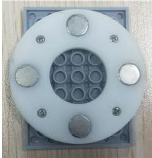
**The fixing plate of the sensor main control board of the M module:** It is used to fix the sensor main control board at the bottom of the M module.
