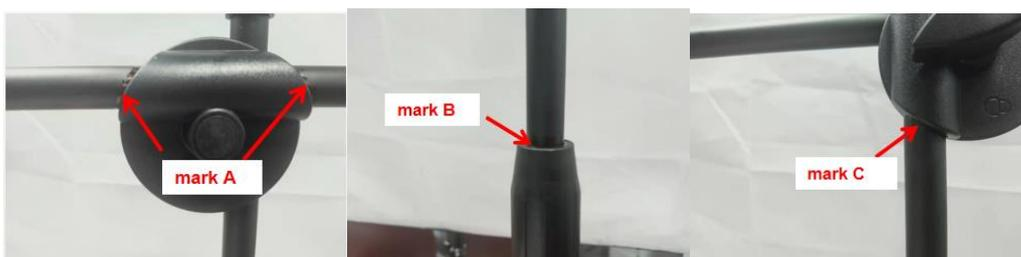
② Fit the bracket parts of the fixed bracket to the marks A, B, and C according to the above figure. The specific effects are as follows:
