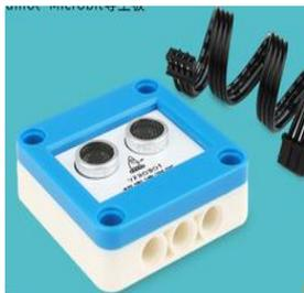
**Ultrasonic sensor:** It is used to detect whether there are obstacles ahead.
