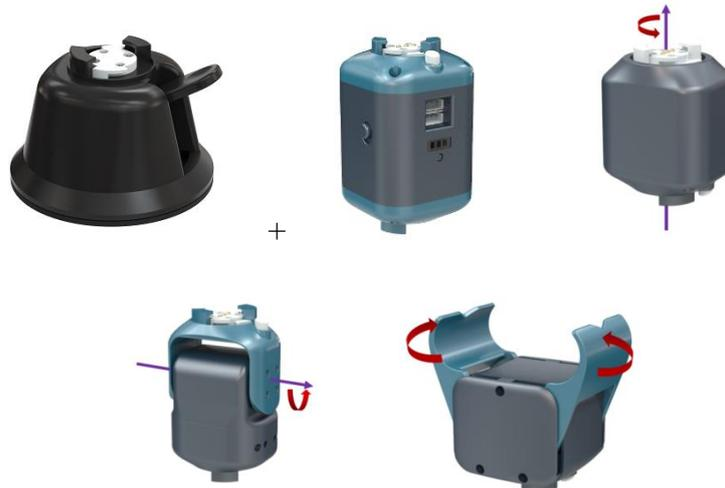
(3) Machine configuration: The robotic arm (F I T T T I G) in this experiment is a five-degree-of-freedom robotic arm, where the numbering sequence is 20, 30, 31, 32, 21, and 40, respectively. Note: 20~29 are I modules, 30~39 are T modules, and 40~49 are G modules. Build as shown below:
