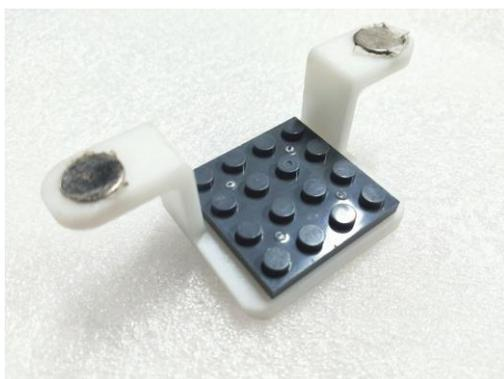
The sensor main control board fixing plate of the M module is used for fixing, and the sensor main control board is fixed at the bottom of the M module.
