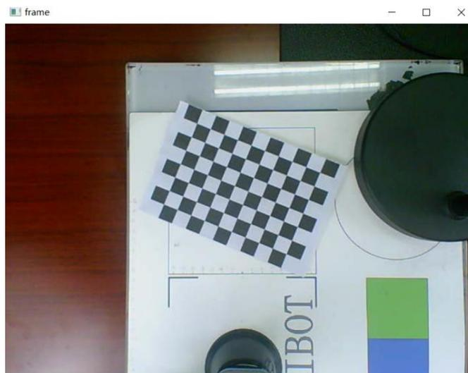
6. Run `3.calibration.py` on the terminal to calibrate the internal and external parameters of the camera;
