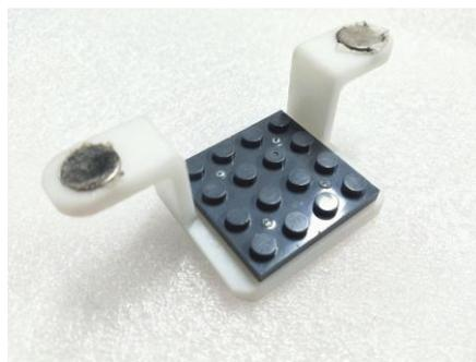
The sensor main control board fixing plate of the M module is used for fixing, and the sensor main control board is fixed at the bottom of the M module.
