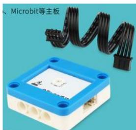
**RGB lights:** It is used to display lights of different colors.
