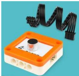
**Sound sensor:** It is used to detect and feedback external sound.
