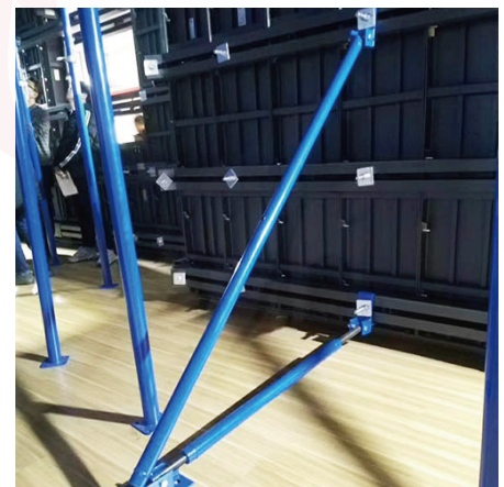
STEEL SHORING ADJUSTABLE W/ BRACING PLATE
