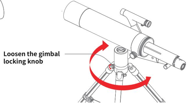
Release the gimbal locking knob and pitch locking armrest to confirm the observation target.
