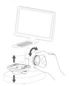
5. Remove the lens cover and put in the observation items (note that the specimen should be facing the eyepiece)
