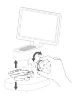
6. Select the multiple to be observed (note that the specimen should be facing the eyepiece)
