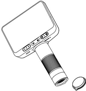
2. Holding the base with one hand, insert the microscope monoblock vertically downward into the mounting hole, paying attention to the rear slot aligned with the mounting hole.
