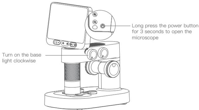
3. Adjust the microscope lift knob, so that the lens barrel is at a relatively suitable height, easy to place the object of observation.
