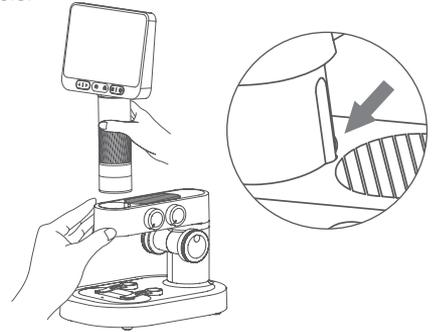
3. Insert to the bottom (Expose the focusing rotary cylinder) .
