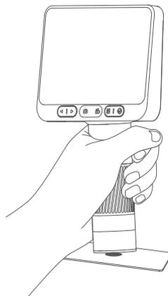
5. The other hand rotate the focus rotating cylinder, observe the screen display, and adjust to the best observation effect.
