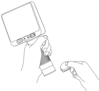
4. Aim the microscope at the object to be observed.
