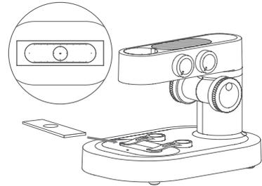
5. Rotate the focus knob, observe the screen display, and slowly adjust to the best viewing (Adjust the viewing height and focal length to achieve different magnifications of viewing.)
