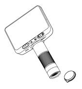
2. Holding the base with one hand, insert the microscope monoblock vertically downward into the mounting hole, paying attention to the rear slot aligned with the mounting hole.
