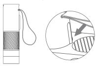
3. Holding the base with one hand, insert the microscope monomer vertically down into the mounting hole.
