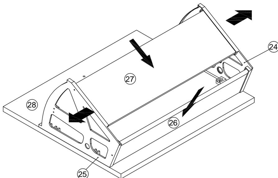
Move the upper part of (24) (25) and put the # 26 # 27 board into the slot
