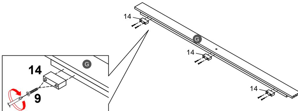
Drawer stopper (14) with lower side rail front (G) by using screw (9).
