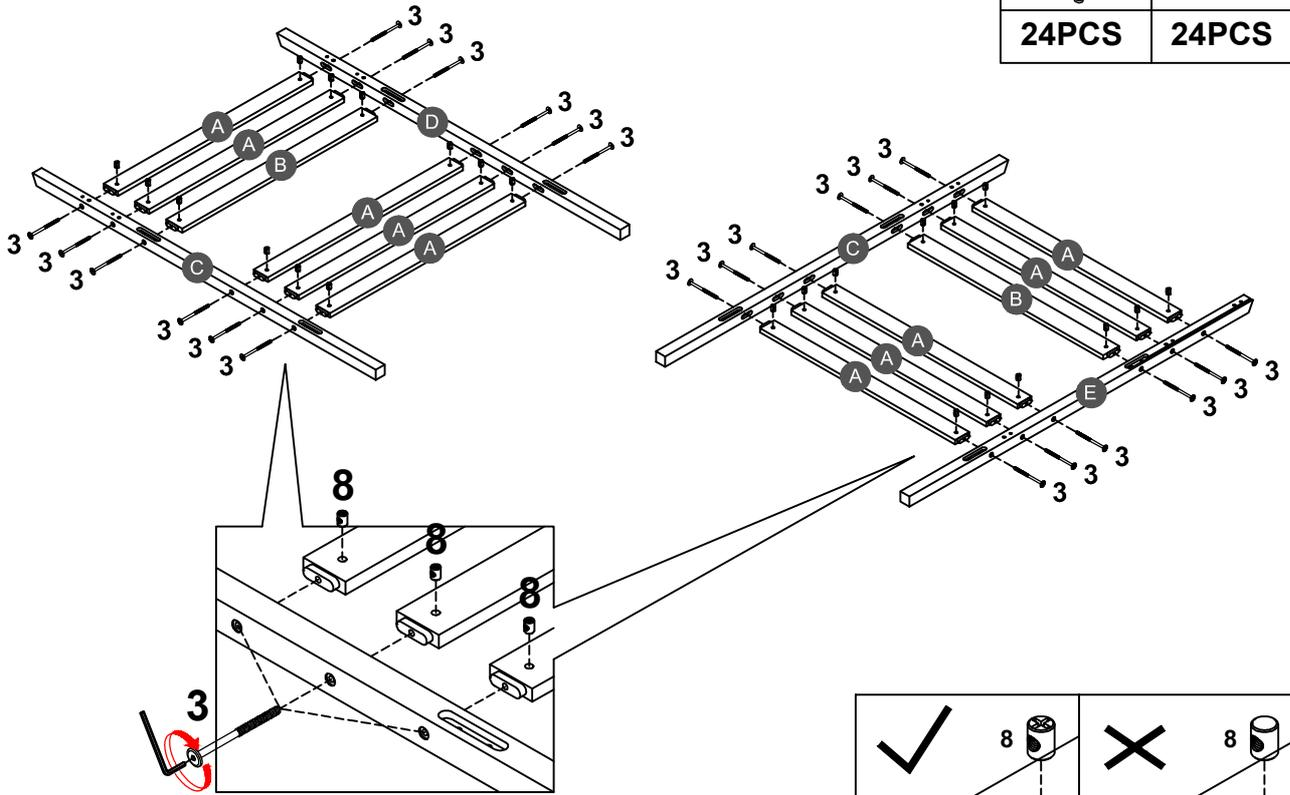
Note: Part 8 will face up with the "x" mark on it, otherwise it cannot be tightened
