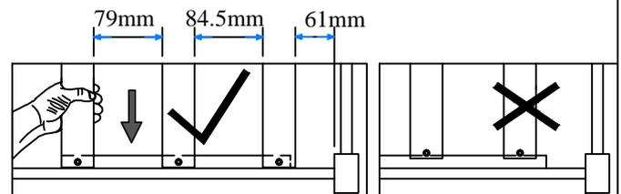
Note: Do not lock the screws of the bed slats to the outermost edge of the bed slats, you need to leave a certain space at the edges, otherwise it will cause the board to break. Do not lock the bed slats on the edge of the wood, please hold firmly before screwing , hold it in place with one hand, then lock the screw.
