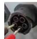
Measuring the voltage between three phases: 402.2V
