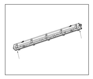
11. Secure lens to housing with lens latches.
