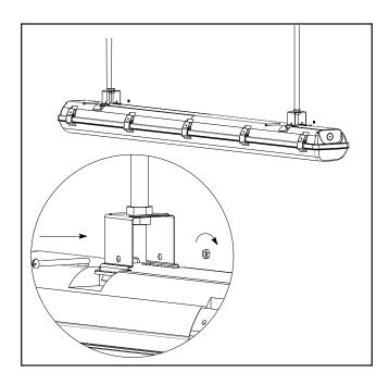
2. Secure mounting clips to housing recesses by firmly pressing them into place until both sides of the clip are secured.
