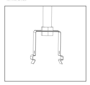
3. Insert the long screw into the hole on the side of the boom bracket and screw the nut on.
