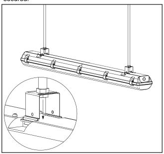
4. Tighten the nut so that the support does not fall off.
