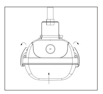
7. Locate safety cable when opening to install fixture body and Snap connect tether to gear tray before making electrical connection as shown in figure.
