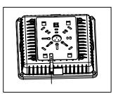
2.Connetc the wires threaded from conduit and canopy,Black wire for Line,White forNeutral, Yellow Green for ground
