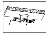
3.Attach the Canopy light with bracket by putting the ring on clips again. Connect the Black wire for line, white for Neutral, Yellow Green for Ground
