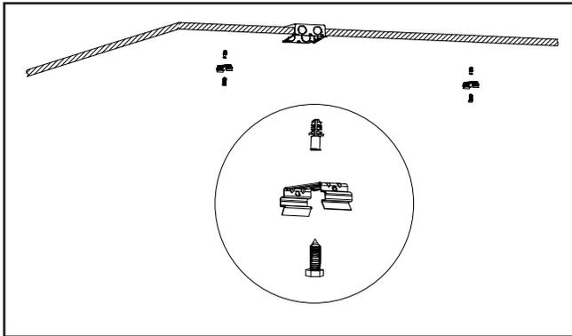
2. Secure mounting clips to housing recesses by firmly pressing them into place until both sides of the clip are secured.
