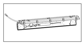
2. Secure mounting clips to housing recesses by firmly pressing them into place until both sides of the clip are secured.
