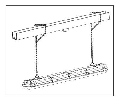
2.Secure mounting clips to housing recesses by firmly pressing them into place until both sides of the clip are secured.Hang fixture from customer supplied chain using V-brackets.
