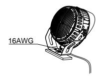
Connect the AC line, AC line for 16 AWG.
