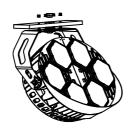
(1)Hold luminaire in place and install bolt, flat washers, and nut to securely fasten the fixture mounting bracket to the mounting structure.
