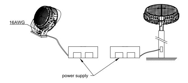
You can take out the power supply from the lamp body, extend the power output line, put the power supply in the power box.
