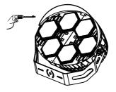
Take the lamp out of the carton and fix the reflective cover as shown in the picture.
