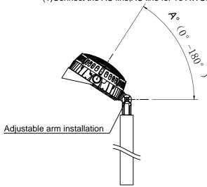
(2)Install the fixture on the pole.
