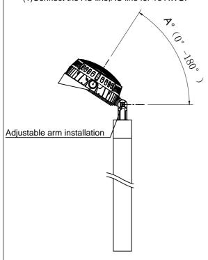
(2)Install the fixture on the pole.
