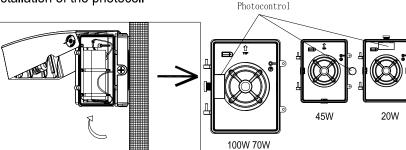
1.Pick a ½" cap of either side of the product and install the photocell according to the picture.
