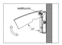
4. Customer adjust the two adjusting screw of the lamp according to their own needs Fixed the angle of the lamp (as shown).
