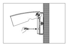
3. After the AC power cord is connected, the upper cover and the lower cover are locked by screws (as shown).
