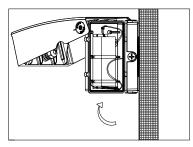
2. The upper cover and the radiator (assembly) are assembled into the shaft hole through the rotating shaft. Connect the AC power line. (as shown in the picture).
