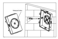
1. Stick the waterproof cotton on the bottom of the lower cover, and the lower cover is fixed on the wall with screws. The light control is assembled to the lower cover of the power supply box. (as shown in the picture)
